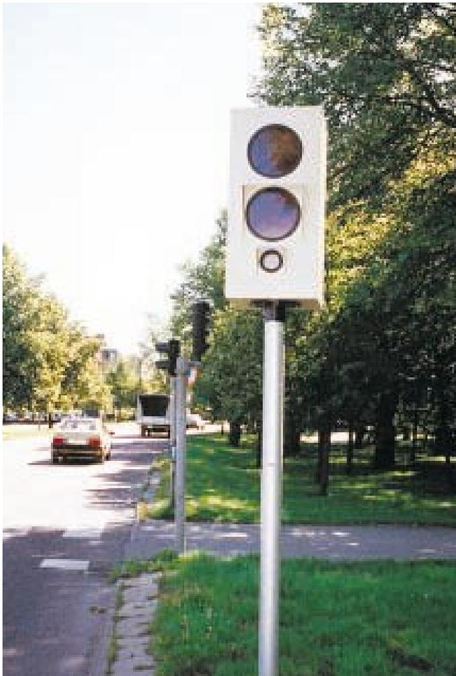
In order to reduce the number of serious accidents on the E4 between Hudiksvall and Iggesund, seven automatic traffic monitoring cameras have been installed in 1998. The equipment includes a radar which gauges the speed of all passing vehicles, which in turn is connected to the camera, which photographs any car exceeding the speed limit.
