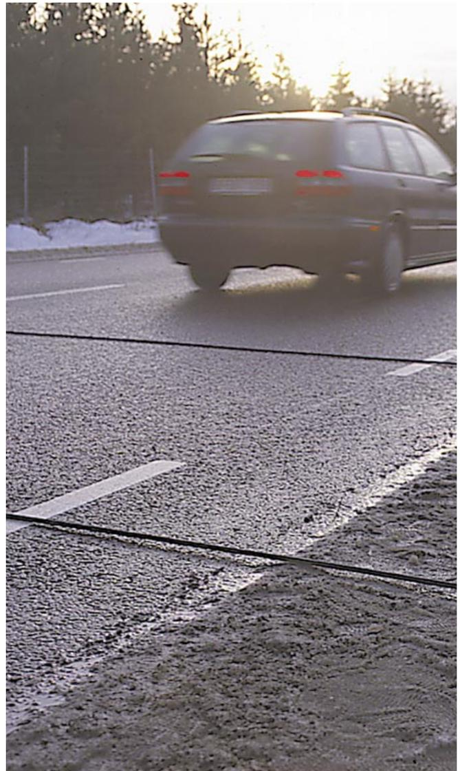
Every day, vehicle mileage, speed, headway and type of vehicle are gauged at some 250 'assessment stations' like this on the road network.
